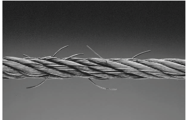
Cable With Broken Wires
